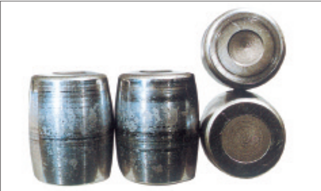
Photo 7-2-3 Part: Convex roller of Photo 7-2-1 Symptom: Round shaped peeling pattern occurs on the center of the rolling surfaces Cause: Poor lubrication
