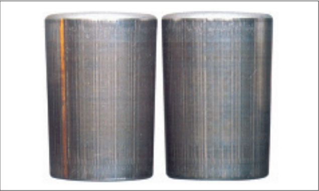
Photo 7-15-2 Part: Tapered rollers in Photo 7-15-1 Symptom: Striped pattern of corrosion occurs on the rolling surface
