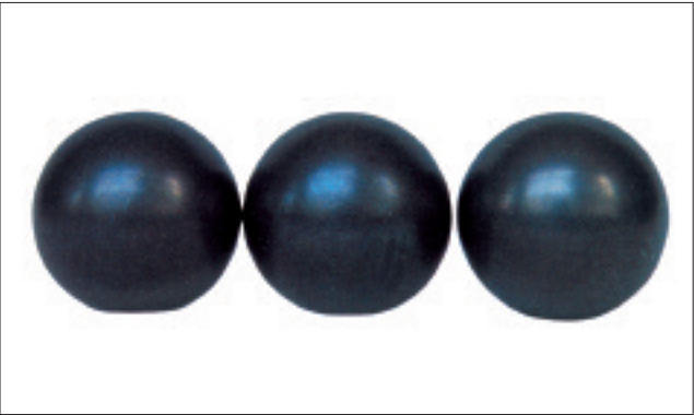
Photo 7-15-4 Part: Balls of a deep groove ball bearing Symptom: Electrical corrosion has a dark color that covers the entire ball surface
