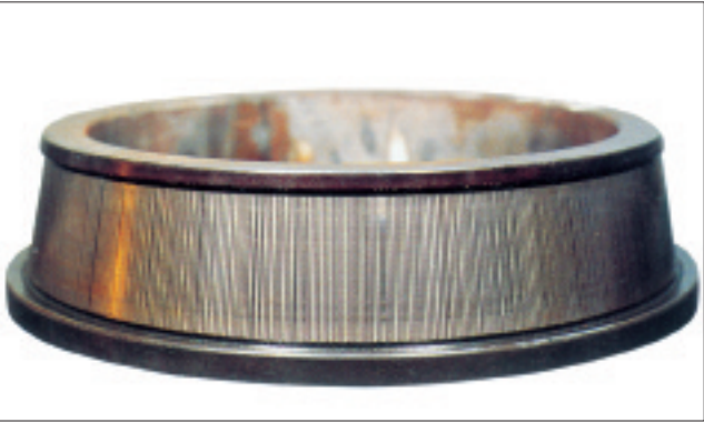
Photo 7-15-1 Part: Inner ring of a tapered roller bearing Symptom: Striped pattern of corrosion occurs on the raceway surface
